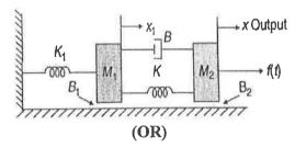
2. (a) Determine the transfer function for the given system.
